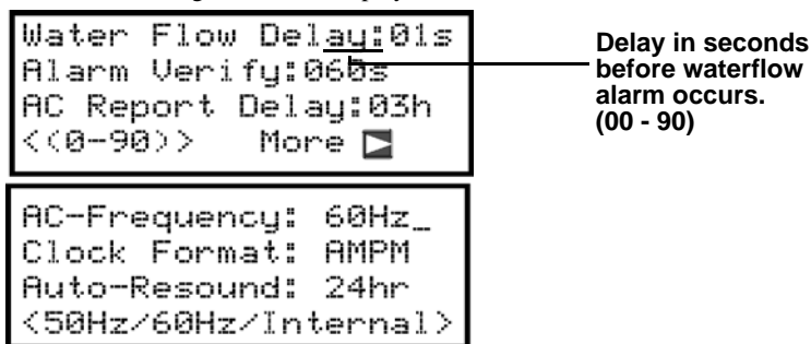
Figure 9.9 Water Flow Delay Programming Screen
